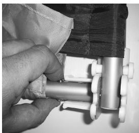
2. Press the spring button to un-lock the tube
