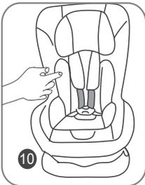
B) Press the seat reclining adjustment handle and pull the seat to the fully reclined position. The fully reclined position required for group 0+ is reached when the red arrow on the side of the back seat lines up with position "4" indicated on the corresponding side of the base and you will hear a "click" as it locks.
